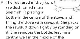
it. She removes the bottle, leaving a sawdust. She places a lid with a hole in the centre over the stove. She puts two bricks on the lid and rests the cooking pan on top. To light the stove, a lit twig is placed in a hole at the bottom of the
